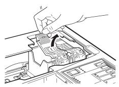
Lift the cartridge out of the printer and dispose of it carefully so any excess ink does not spill. Do not take the used cartridge apart or try to refill it.
